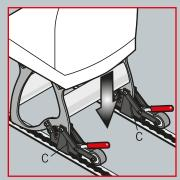
Lower the rest of the seat into the tracking.
