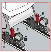
Close handles B to lock the chair in its new position. The safety bolts (A) should rest in their lower position.
