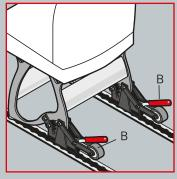
Rest on tracking and ensure handles B are unlocked by pointing away from the chair as shown next to the left. If not please unlock them using the instructions in the next section on the right.
