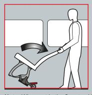
Using the wheels as a pivot point, lean the seat backwards out of the floor tracking.
