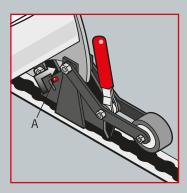
Lift safety bolt A to its upper position.
