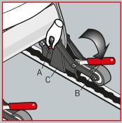
While holding safety bolt A in its upper position pull handles B away from the Fitting C to unlock. Repeat on other leg.
